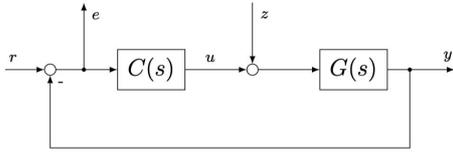
$$\begin{aligned} r \rightarrow y & \quad TF = CG / (1 + CG) \\ z \rightarrow y & \quad TF = G / (1 + CG) \\ r \rightarrow e & \quad TF = 1 / (1 + CG) \\ z \rightarrow e & \quad TF = -G / (1 + CG) \end{aligned}$$
