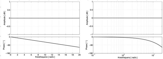
$$\angle G(j\omega) = \frac{(T - T_t) - T}{T} \cdot 360^\circ = -\frac{T_t}{T} 360^\circ = -T_t f 360^\circ = -T_t \frac{\omega}{2\pi} 360^\circ$$
